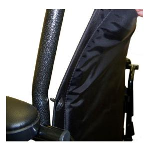
4. Slide the mounting plate of the STDS834 between the back post and the back upholstery.
